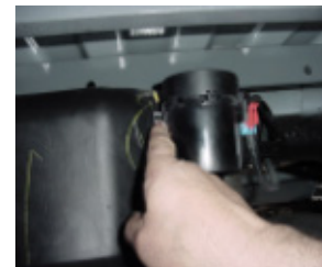
Figure C2, Step 2: Disengage the locking pin.
