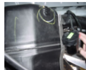
Figure C4, Step 4: Install Center Section, Step 5: Replace fuel valve to bracket on fuel tank after installation.
