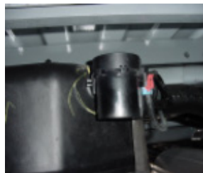
Figure C1, Step 1: Locate the Fuel Valve.
