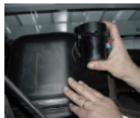
Figure C3, Step 3: Slide fuel valve from bracket.
